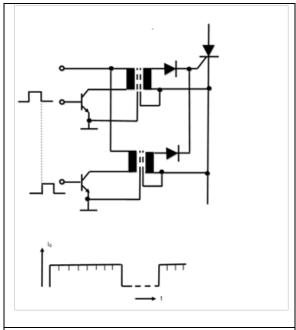
Figure 5. Interleaved pulses
